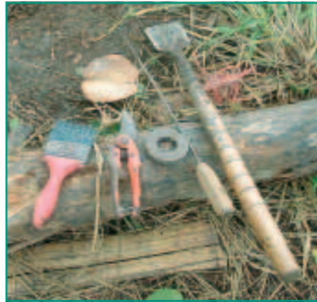
Figure 16. A CMAC deminer's signal-investigation tools. Both the prodder and the CMAC trowel were locally made and details varied. A "doughnut" speaker magnet is in the centre of the picture.
