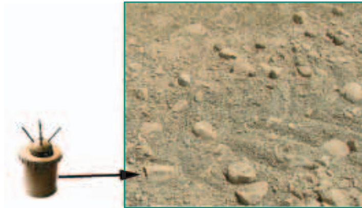
Figure 10. The body of an unexploded V69 is crushed into the tracks of a flail.
