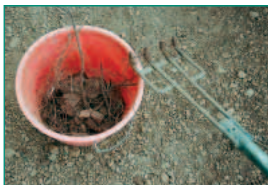
Figure 4. A four-tine adaptation of the Harrow-rake developed by DDG.
