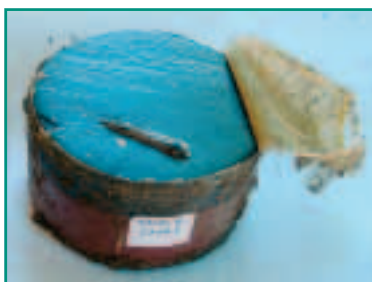
Figure 27. The damage to the top of this surrogate GYATA-64 was not visible before the witness plate was peeled away.
