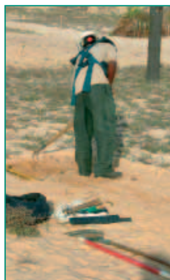
Figure 1. Harrow-rake in use showing the long tines. Metal Brush-rake in foreground.
