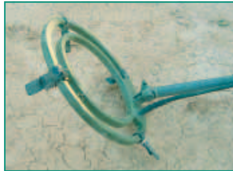
Figure 6. Head of Schiebel detector with guiding ties.
